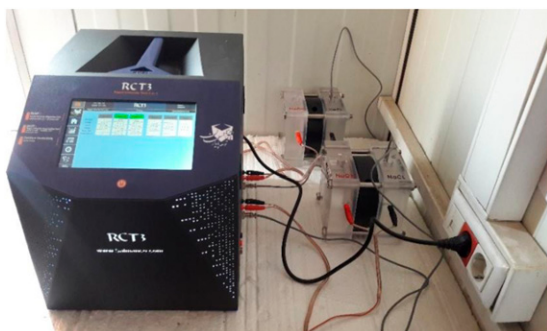
Figure 2. The rapid chloride penetration test setup.
