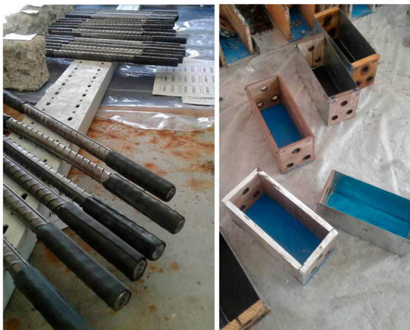
Figure 3. The steel rebars and molds to constructing corrosion test specimens.
