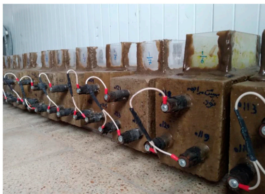
Figure 4. The constructed corrosion test specimens.
