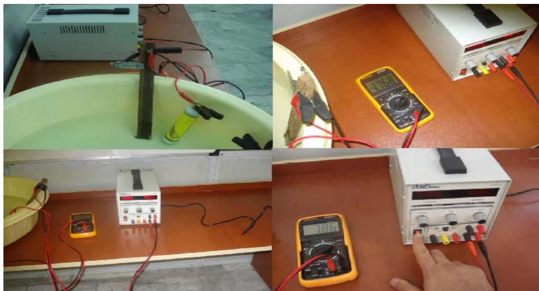
Figure 2: Photographs of the mounted CP system for the net polarization monitoring
